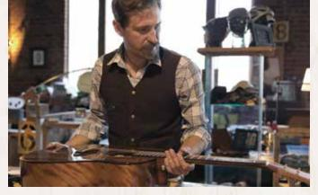
4. If your bridge truss is in need of adjustment, tighten (clockwise) or loosen (counterclockwise) the bolt on the front of the wood block (it is visible through the sound-hole). A very small turn of the bridge truss bolt can be enough to return the rod to proper tension, so make adjustments in very small increments and check tension after each turn of the bolt.
